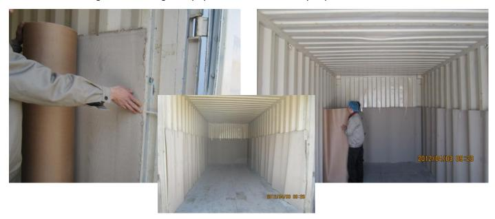
3. Container floor to be covered with two corrugated papers with a 20cm overlap. Fold excess paper(30cm) from side to cover the lashing rings/bars(located on the longitudinal rails and corner posts)
